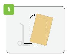
Tip the box slightly forward and push the platform of the sack trolley under it.
