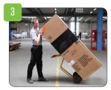
Tip down the box until it is balanced and the weight is resting on the trolley wheels.
