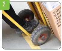
Block the sack trolley with one foot to prevent it from moving backwards.
