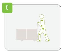
Stop by pushing the handle in upright position and use your body to push back – or lower the pallet.
