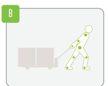
When the pallet truck is in motion, turn around and pull the pallet behind you.
