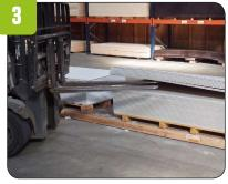
Use one fork to slightly lift the stack from the underlying plates.
