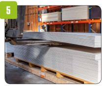
Now you can squeeze the forks in between the required number of plates and the rest of the stack and lift them clear of the stack.
