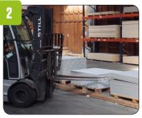
Separate the plates by pushing the wedge further in using the forks of the truck.
