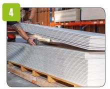
Move the wedge to the centre and lower the stack of plates until they rest on the wedge.
